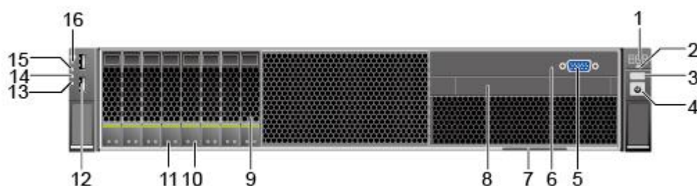
Figure 4-4 Front panel of the RH2288 V3 with eight hard disks
